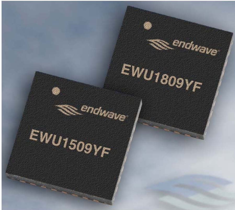
Fig 5. Millimeter-wave monolithic microwave integrated circuits (MMICs) like these products from Endwave are becoming more common. Made with gallium-arsenide (GaAs) pHEMT technology, these upconverters include mixers, local oscillators, doublers, and variable gain RF amplifiers. The EWU1509YF covers 10 to 15.4 GHz, while the EWU1809YF covers from 17 to 24 GHz.
