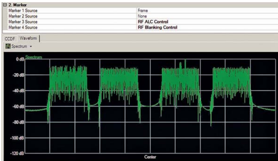
Fig 3. The spectrum of the LTE-Advanced configuration includes four non-contiguous 20-MHz carriers, as shown with Agilent Technologies' LTE-Advanced signal generation software.
